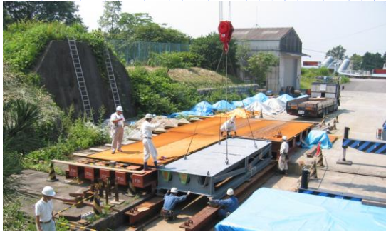
Specimen is installed into loading stage
